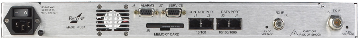
Figure 4-2 MDX420 Satellite Gateway Rear Panel
